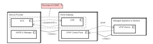
Fig. 1: A typical autonomic operations management architecture using CWMP
