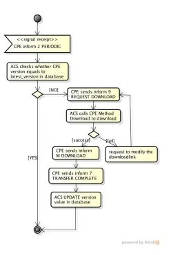
Fig. 3: Supporting self-diagnosing tasks: Check and upgrade a deployment unit
