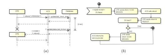
Fig. 4: Supporting self-diagnosing tasks: (a) diagnose CPE (b) diagnose and recover DU
