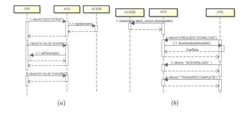
Fig. 2: Supporting self-deployment tasks: (a) setup a newly installed system (b) install a new deployment unit
