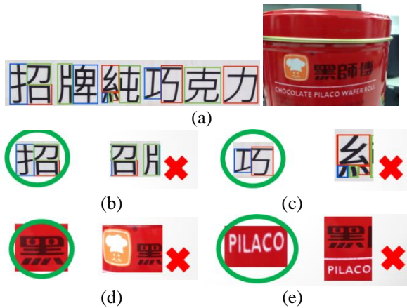
Figure 19. Examples illustrating the criteria for text candidate linkage. (a) Source images (b) Spacing criteria (c) Difference of width and height (d) Difference of mean of grayscale (e) Difference of mean of stroke width
