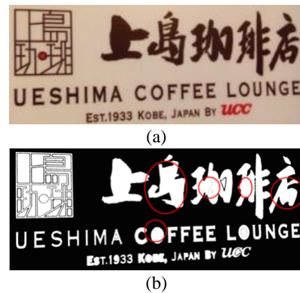
Figure 10. MSER detection. (a) Original image (b) MSER detection result. The areas circled in red show incomplete and ambiguous results.
