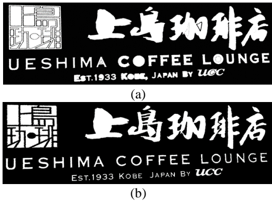
Figure 13. (a) MSER detection result (b) Merging MSER and Canny detection results.
