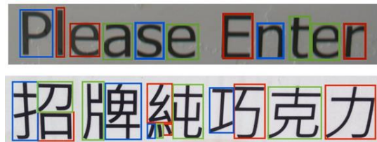
Figure 15. Characters marked by merging connected components.
