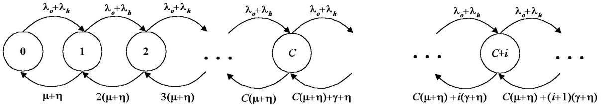
Figure 3. The state transition diagram for the MFIFO scheme.
