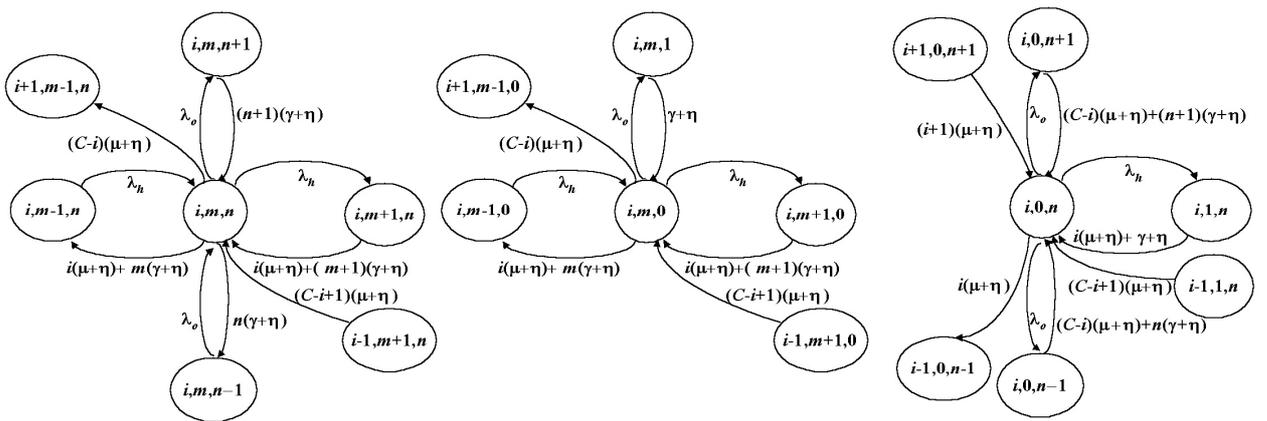
Figure 6. The state transition diagram for the states where  $i : (C - i) \leq w$ .
