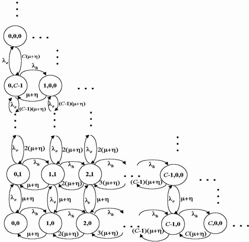
Figure 5. The state transition diagram for the states with free channels.
