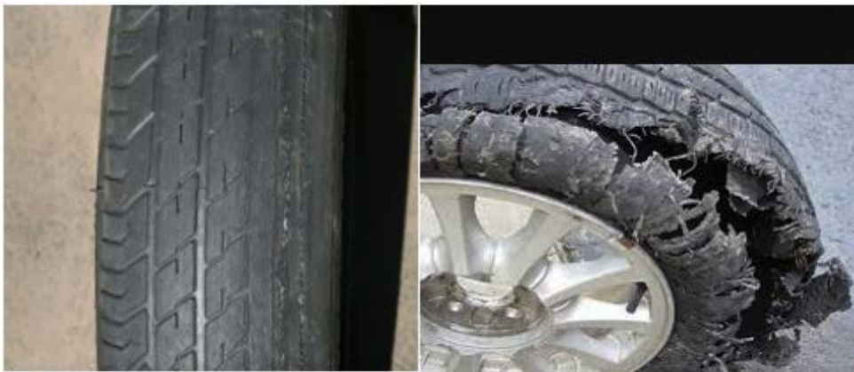
Figure 7: Tyre burst due to lack of wheel alignment and balancing
