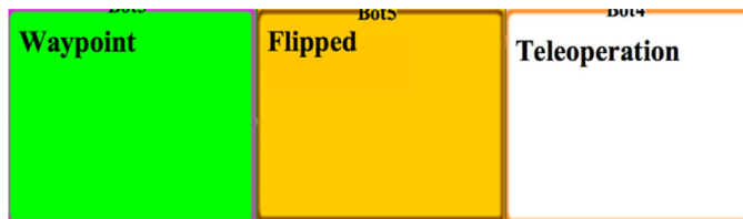
Fig. 3. Status panel: Green color represents a robot is working appropriately; yellow color represents a robot is encountering problems; white color represents a robot is under manually controlled.
