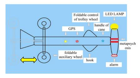
Figure 2. IoT smart cane design
