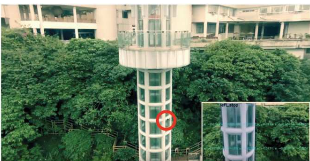
Figure 9. Image taken from another UAV to record the scanning UAV (red circle), the lower right image shows the processed histogram
