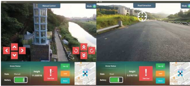
Figure 2. Ground control station screenshots in manual mode (left) and road detection following with crosshair (right)
