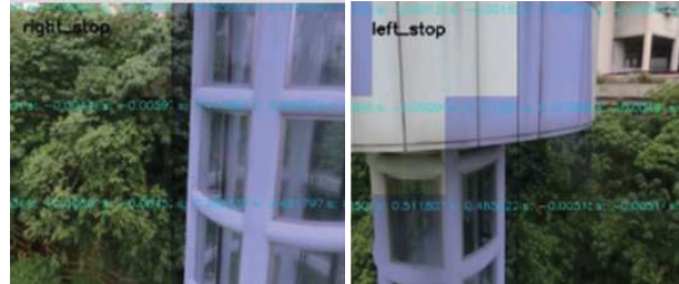
Figure 6. The left image shows the UAV is on the left edge as histogram detects the target on right part, the right image shows the UAV is on the right edge determined by the score left larger than right in purple color
