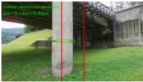
Figure 1. Both lateral deviation and orientation deviation are measured in camera image
