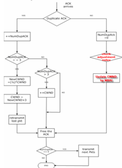
Figure 3.3 : Flowchart of the procedure for TCP Muzha upon receiving an ACK
