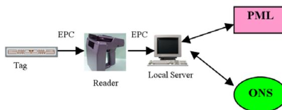
Figure 2: RFID ONS structure
