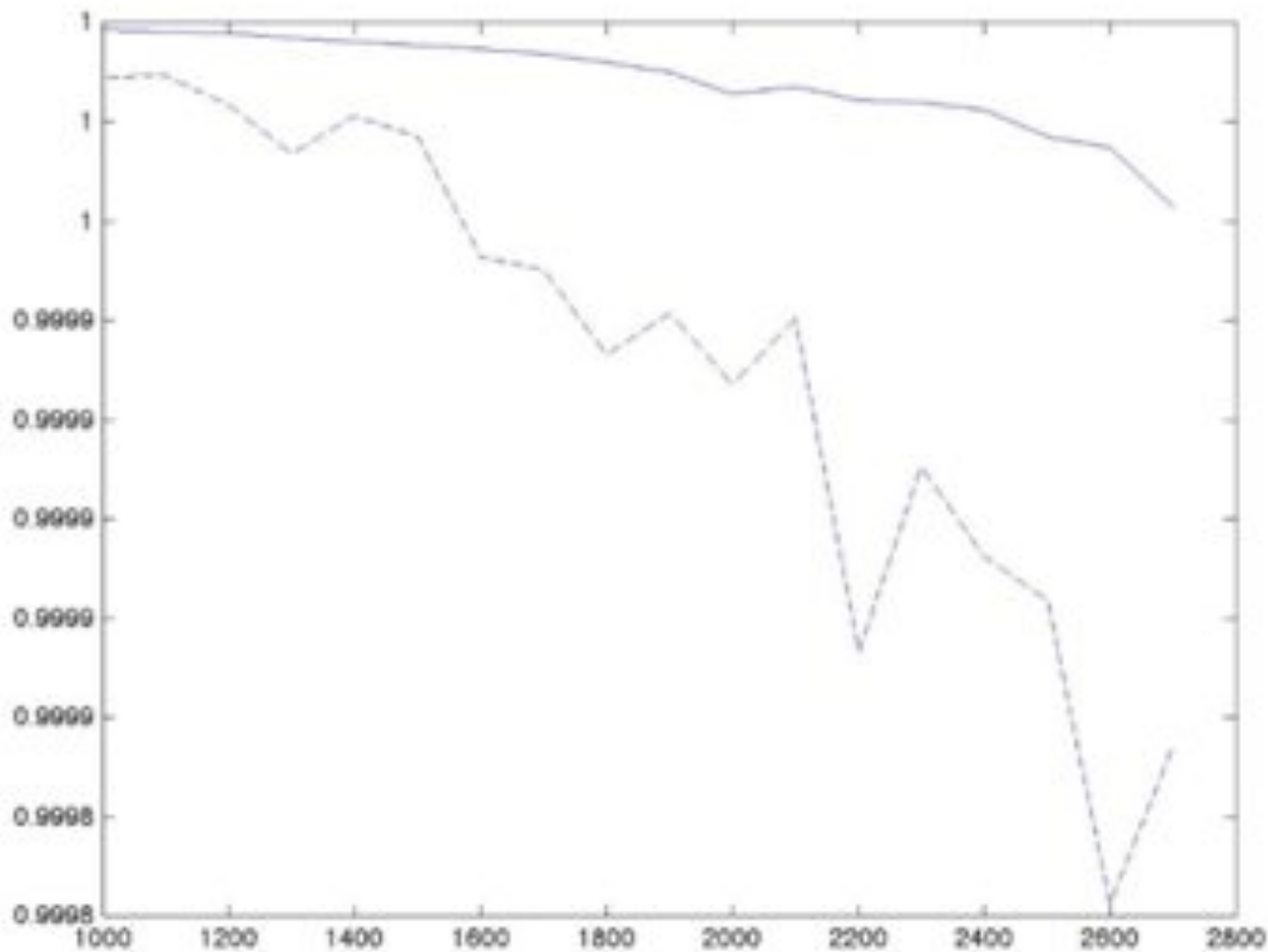
Figure 4. The orthogonality between approximated SVD and true SVD. The solid line is a^{(t)} and the dashed line is b^{(t)}
