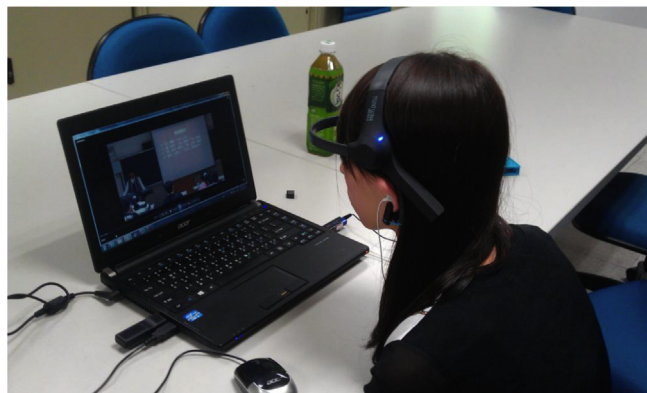
Fig. 4. The experimental scene of a learner who simultaneously wore a Mindset earphone and an emWave stress detector to assess sustained attention and emotion while performing an autonomous online learning by video lecture.
